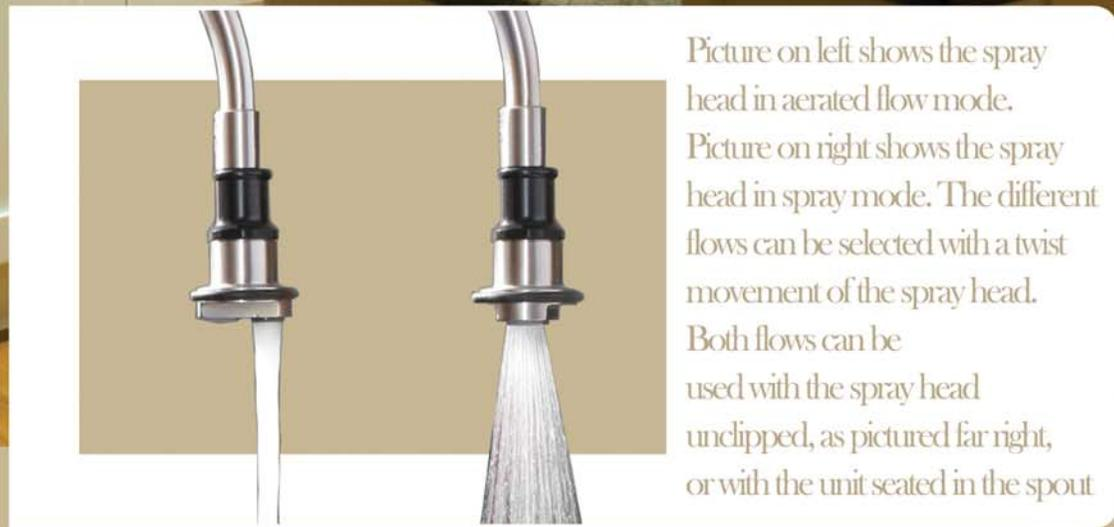
Picture on left shows the spray head in aerated flow mode. Picture on right shows the spray head in spray mode. The different flows can be selected with a twist movement of the spray head. Both flows can be used with the spray head unclipped, as pictured far right, or with the unit seated in the spout
